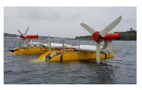
i Minesto's Deep Green device comprises a turbine integrated with a wing, which is tethered to the seabed and operates in a manner similar to an airborne kite.
